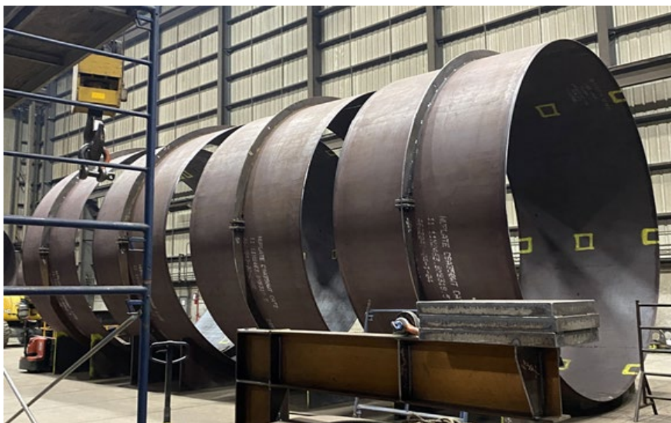
Figure 3: Fabrication (Ring Segments) – Cans 4 and 10
