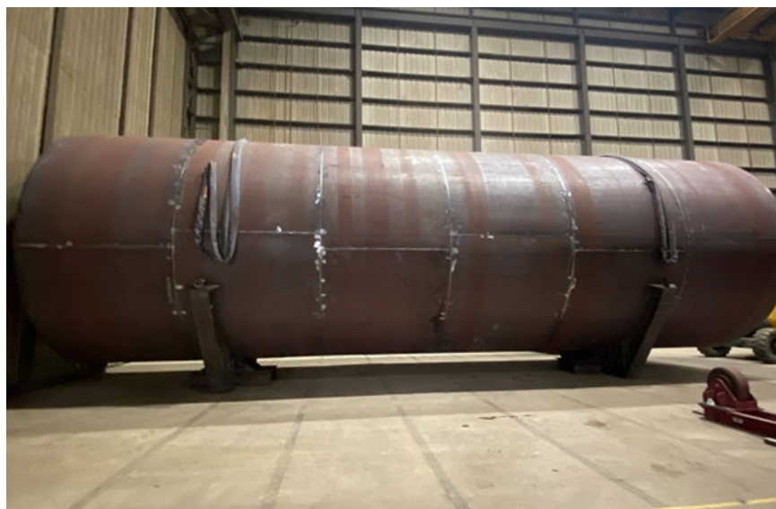
Figure 4: Fabrication (Complete and awaiting Blast and Paint) – Can 8
